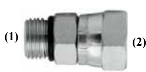
(1) ORB male, (2) NPSM swivel SAE# 140157 Parker 0507 Aeroquip 2066 (Reversed) Weatherhead 9315
