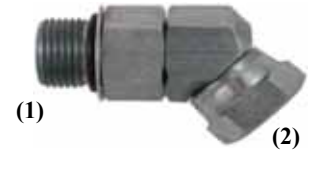
(1) ORB male, (2) NPSM swivel SAE# 140357 Parker 3507 Aeroquip 2067 (Reversed) Weatherhead 9365
